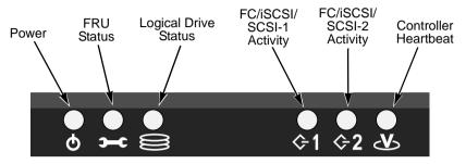
Figure 14. VTrak M500f/i/p front panel LED display
